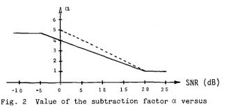
the SNR. is smaller for higher SNR inputs. We then decid
